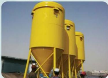
Portable Silos For Plaxit / Rak Fix / Dubai Plaster
